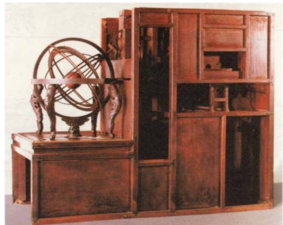
Astronomical Instruments in Korea. Fig. 6 Armillary clock in the Museum of Korea University, Seoul.
